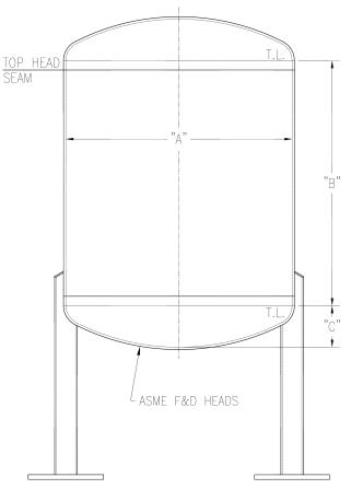
Note: The capacity (In Liters) volume level is figured at the "Top Head Seam".
