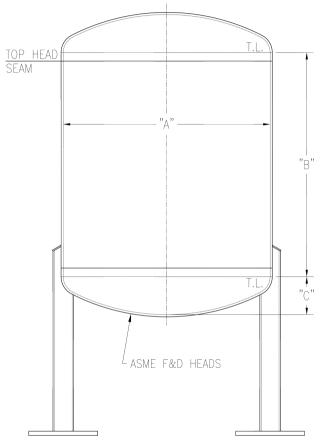
Note: The capacity (In Gallons) volume level is figured at the "Top Head Seam".
